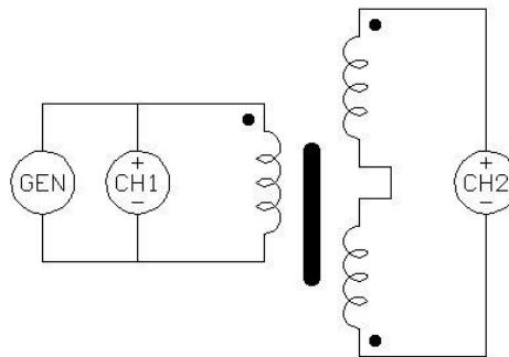
Select 'Vector Voltmeter' mode, and using the SETUP menu select 'LVDT diff' as the parameter. Enter the electrical stroke of the LVDT in meters as the scale factor (if required). The in-phase component of the secondary is computed by DFT analysis at the fundamental frequency. The displacement is computed as:
