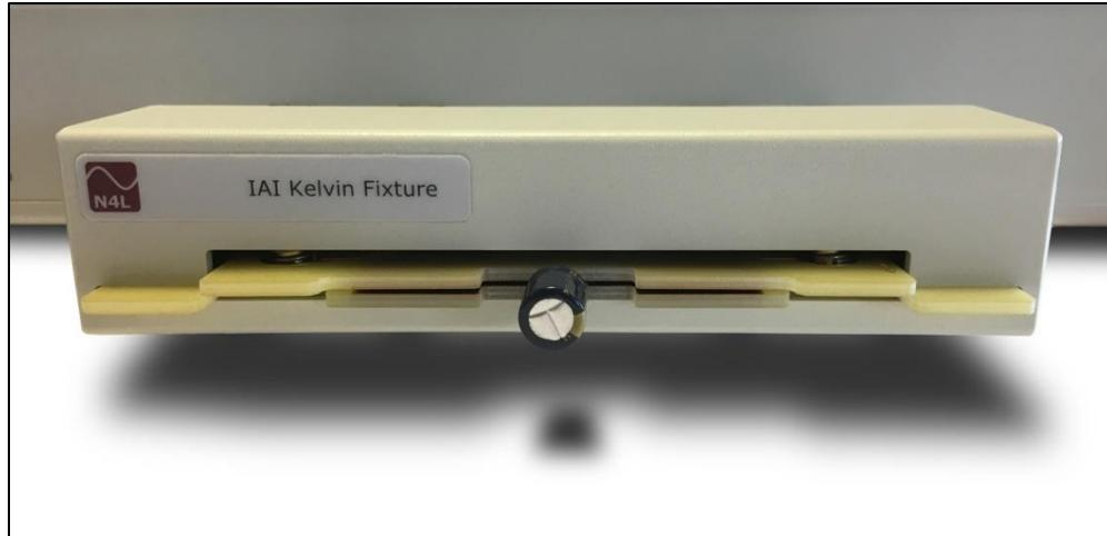
**A convenient 4-wire connection fixture suitable for a variety of components**
