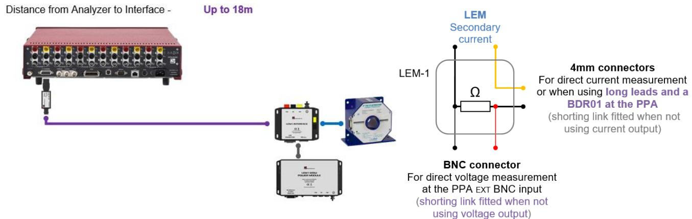
An additional advantage of this connection technique for applications involving a large distance between the measurement instrument current transducer, is that the long cable length uses coaxial wire rather than multicore DSUB to DSUB cable, so there is superior resilience to residual electrical noise while also being more flexible.
