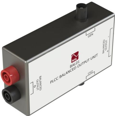
Power Line Carrier Communications balanced output unit designed for use with the SLM3505 Selective level meter
