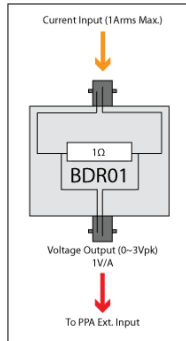
The BDR01 series shunt provides an accurate current sensing solution for current transducers/transformers outputting a current signal, the shunts feature BNC input and Output connectors.
